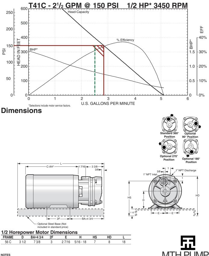
All dimensions in inches. May vary ± ¼ inches. Not for construction purposes unless certified. \*See motor dimensions for "C-AH" dimension
